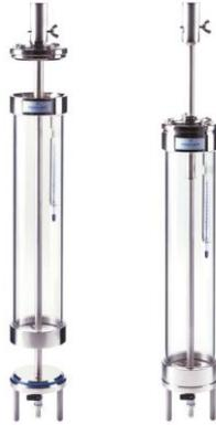
*Figure 3: Ruttner sampler or a closable PVC cylinder that can be lowered and closed in certain depth; sample is taken up on-board the vessel.*
